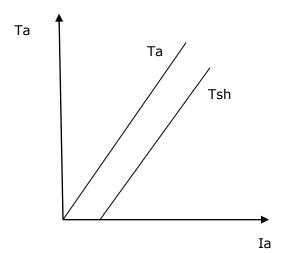
As the load increases, armature current increases and torque produced increases proportional to the square of the armature current upto a certain limit.
