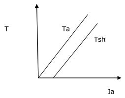
Now, if shaft torque is plotted against armature current, it is known that shaft torque is less than the armature torque and the difference between the two is lasts torque  $T_{\rm L}$ .
