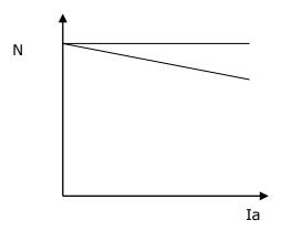
The drop varies from 5 to 15% of full-load speed, being dependent on saturation, armature reaction and brush portion Hence, the actual speed curve is slightly dropping as shown by the dotted line.
