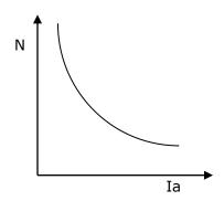
With increased  $I_a$ ,  $\phi$  also increases Hence, speed varies inversely as armature current. When load is heavy,  $I_a$  is large. Hence speed is low (this increases  $E_b$  and allows more armature current to flow). But when load current and hence  $I_a$  falls to a small value speed becomes dangerously high.
